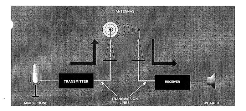
There are several different types of transmission lines. Each type of line has different properties that affect transmission: the bandwidth, the attenuation, and the noise or interference.
