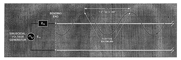
An important characteristic of a transmission line is its **electrical length**,  $l_{\lambda}$ . The electrical length is the ratio of the actual physical length of the line to the wavelength of the signal it carries.
