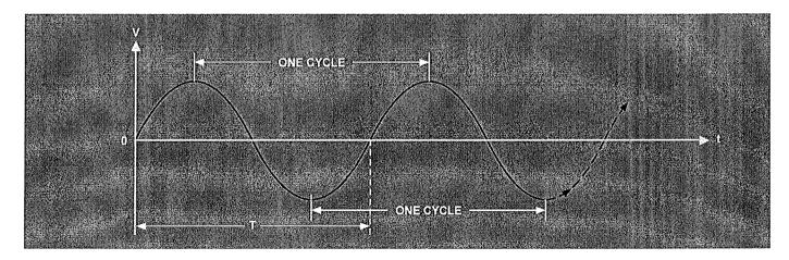
In the context of transmission lines, the variation of a sinusoidal voltage traveling down a line is usually considered as a function of distance rather than time.
