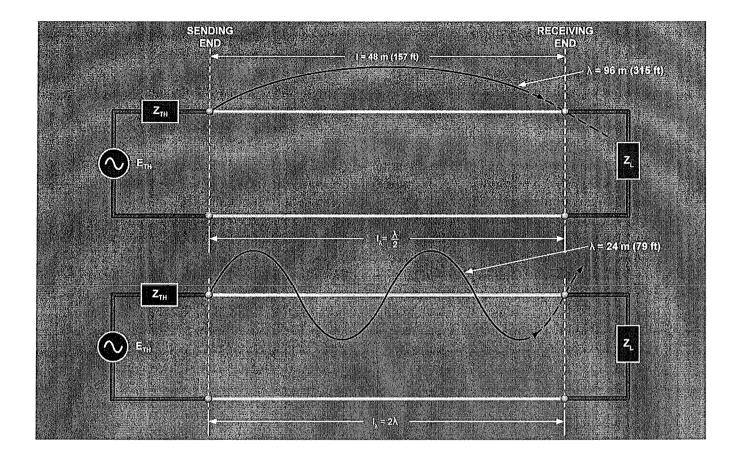
The electrical length of a line (rather than its actual physical length) determines whether the line is short or long with respect to the frequency of the signal it carries.
