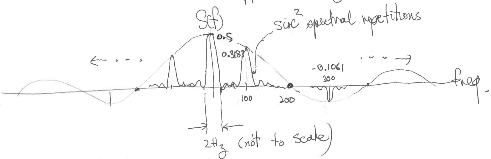
b) The spectrum of a sinusoid  $c(t)$  is simply (at 100 Hz) (1)
