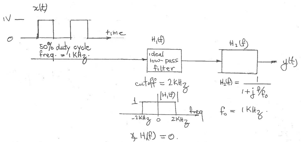
Figure 2: Block Diagram for Q2.
