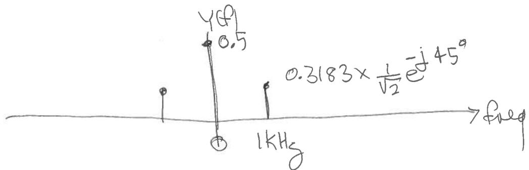
Now we transform  $Y(f)$  into the time domain. The spike at  $0\text{Hz}$  is a DC signal with value 0.5V. The spikes at  $\pm 1\text{KHz}$  transform into a  $\cos(\cdot)$  with amplitude
