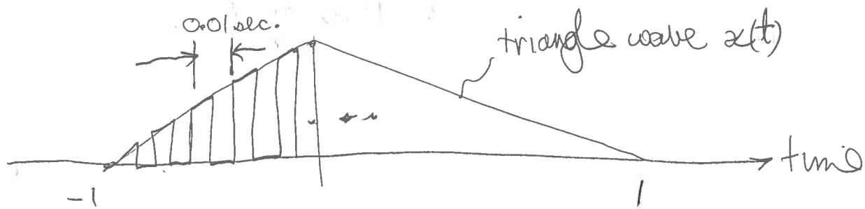
$x(t)$  is formed in the time domain by multiplying  $sq(t)$  with the triangle wave  $x(t)$ . Therefore the spectrum  $S(f)$  is the convolution in freq. of  $X(f)$  with  $Sq(f)$ .
