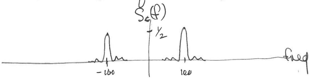
Thus  $S_c(f)$  may be obtained from  $S(x)$  by low-pass filtering (with a cutoff e.g. at  $20.8 \text{ Hz}$ )
