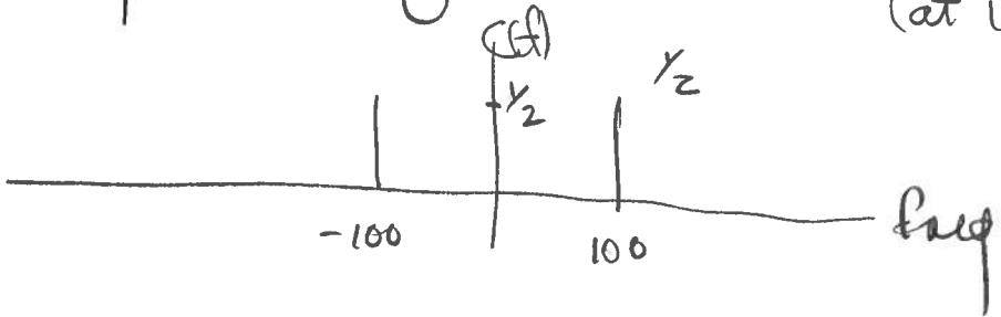
∴  $S_c(f)$  when  $x(t)$  is multiplied by a sinusoid (instead of a square wave) will look as follows
