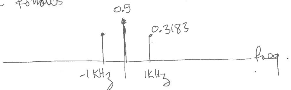
$$\text{At } f=1\text{KHz, } H_2(f) = \frac{1}{1+j} = \frac{1}{\sqrt{2}} e^{-j45^\circ}$$
