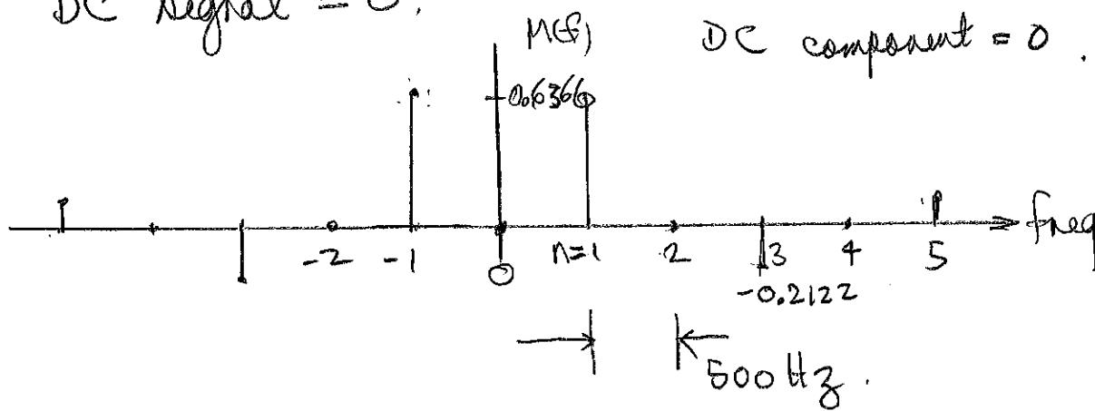
∴ the modulated AM wave has a spectrum as follows: [from (1)]
