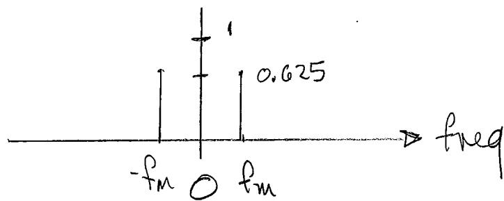
This is equivalent to the message + a DC component. The DC component can be removed by a blocking capacitor to recover the msg.
