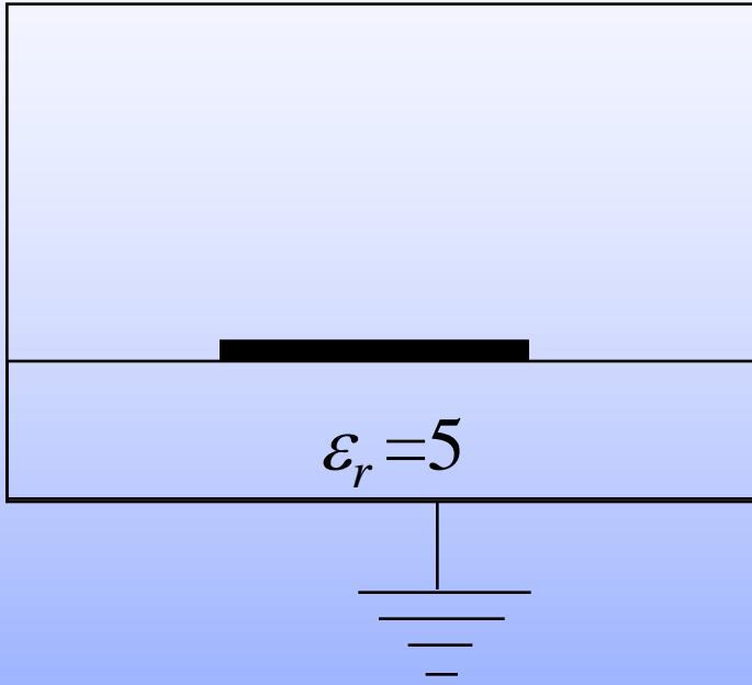
Find the capacitance and the characteristic impedance for the shown shielded microstrip line using the finite element method
