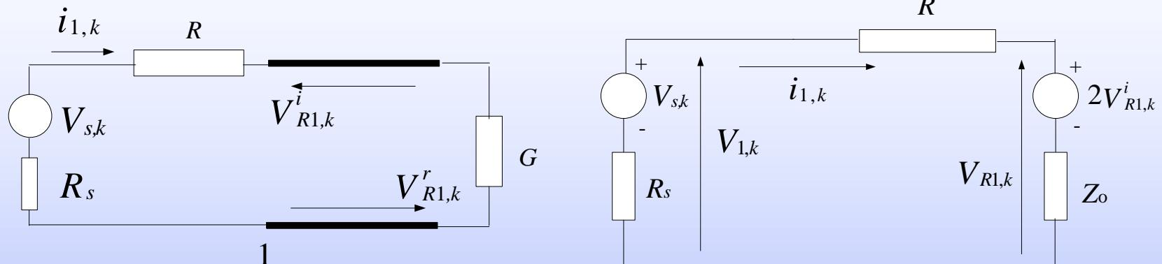
$$i_{1,k} = \frac{V_{s,k} - 2V_{R1,k}^i}{R + R_s + Z_o} , \quad V_{R1,k}^i = 2V_{R1,k}^i + i_{1,k} Z_o$$
