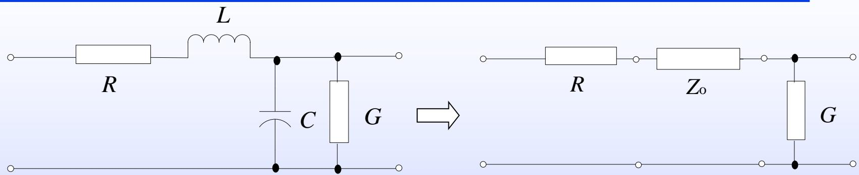
$$Z_o = \sqrt{\frac{L_d}{C_d}} = \sqrt{\frac{L}{C}}, \quad \Delta t = \frac{\Delta x}{u} = \Delta x \sqrt{L_d C_d} = \sqrt{LC}$$
