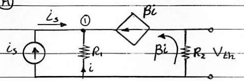
$$\text{KCL at node 1} \quad i_s + i + \beta i = 0 \quad \therefore i = -\frac{i_s}{1+\beta}$$
