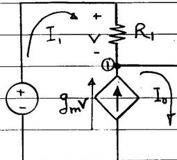
$$\therefore I_o = \frac{V_s}{R_1} + g_m V_s = \left( \frac{1}{R_1} + g_m \right) V_s \Rightarrow I_o = 0.025 V_s$$
