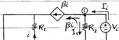
$$\text{KCL at node 1} \quad I_i = I_1 = V_i / R_2 \Rightarrow R_{th} = R_2 = 39 \Omega$$
