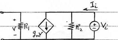
$$\therefore V_i = R_2 I_i \Rightarrow R_{th} = R_2 = 1 \text{ M}\Omega$$
