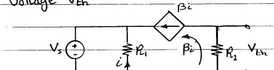
$$\text{but } i = -V_s / R_1 \Rightarrow V_{th} = +\frac{\beta_i R_2}{R_1} V_s = 58.5 V_s$$
