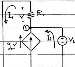
$$\& \quad I_i = V_i / R_1 \quad \therefore \quad I_i = \left( \frac{1}{R_1} + g_m \right) V_i$$
