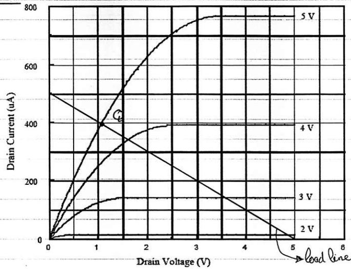
For the loadline :  $V_{GS} = 0 \Rightarrow I_D = \frac{V_{DD}}{R} = 0.5 \text{ mA}$
