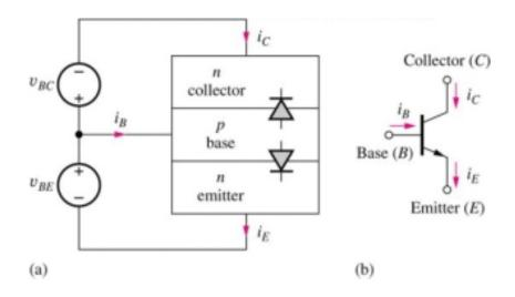
Bipolar Junction Transistors Small-Signal Modeling and Linear Amplification - BJTs
