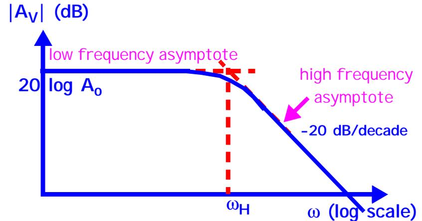
Low pass  $A_V(s) = A_o \cdot \frac{\omega_H}{s + \omega_H}$  ; high-pass amplifier  $A_V(s) = A_o \cdot \frac{s}{s + \omega_L}$
