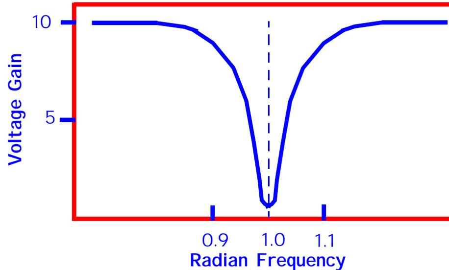
$$A_V(s) = \frac{A_o \cdot (s^2 + \omega_o^2)}{s^2 + s\frac{\omega_o}{Q} + \omega_o^2} . \text{ Write expressions for mag. \& phase?}$$
