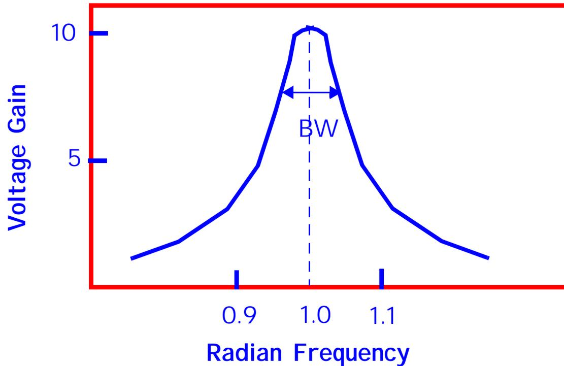
$$Q = \frac{\omega_0}{\omega_H - \omega_L} = \frac{f_0}{f_H - f_L} = \frac{f_0}{BW}$$
