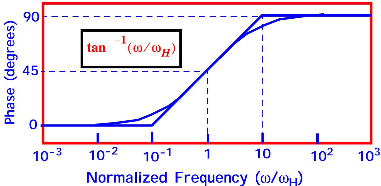
Example: Sketch the bode diagram for the transfer function
