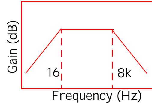
$$|A_o| = 20 \cdot \log(400) = 52.0 \text{ dB}; \quad f_L = \frac{100}{2\pi} = 15.9 \text{ Hz}; \quad f_H = \frac{50000}{2\pi} = 7.96 \text{ kHz}$$
