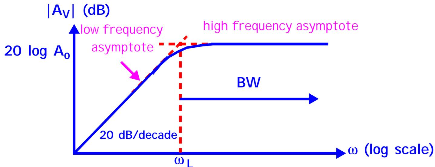
$$\angle A_V(j\omega) = \angle \frac{A_o j\omega}{j\omega + \omega_L} = \angle A_o + 90^\circ - \tan^{-1}\left(\frac{\omega}{\omega_L}\right)$$
