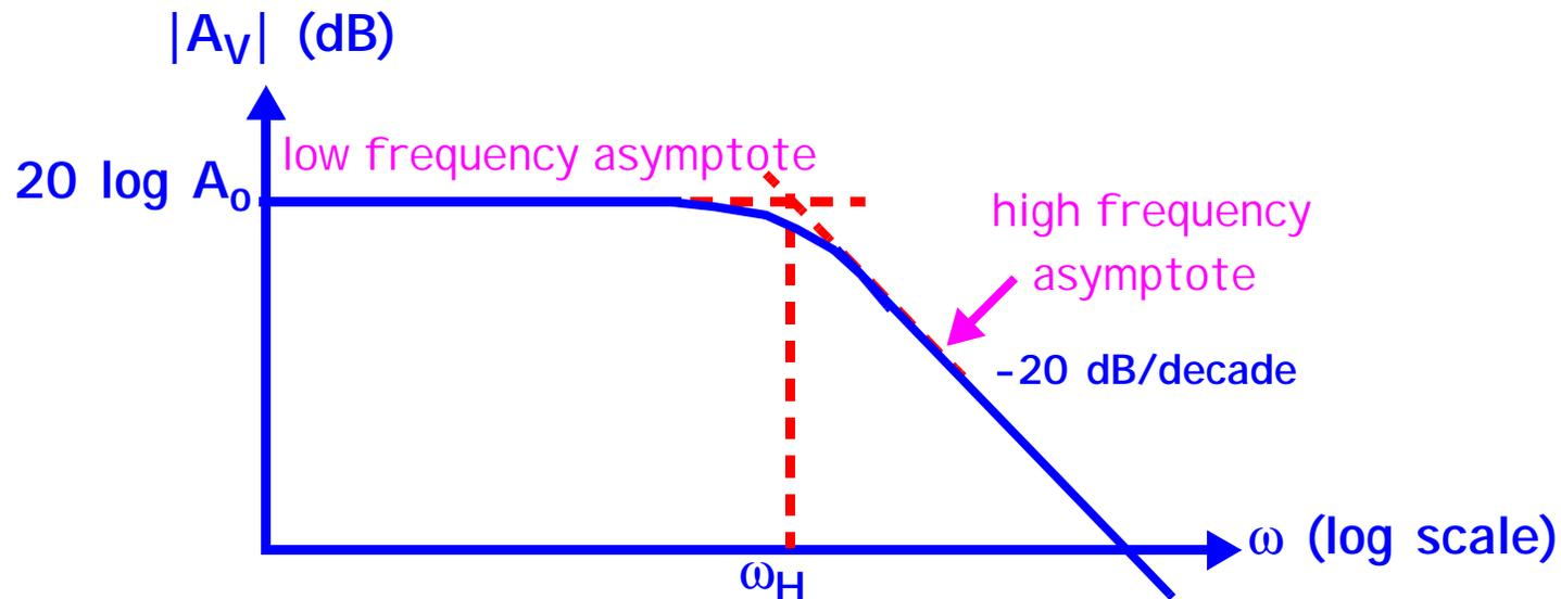
$$A_V(s) = A_o \cdot \frac{\omega_H}{s + \omega_H} ; |A_V(j\omega)| = \frac{|A_o \omega_H|}{\sqrt{\omega^2 + \omega_H^2}}$$
