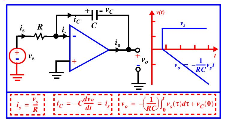
Used in function generators (triangular and sawtooth wave generators), active filters, ADC and analog control.
