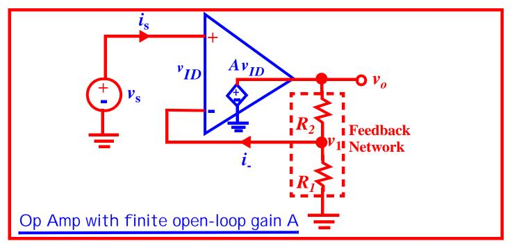
$$v_o = A \cdot v_{id} = A \cdot (v_s - v_1); v_1 = \frac{R_1}{R_1 + R_2} \cdot v_o = \beta \cdot v_o.$$
