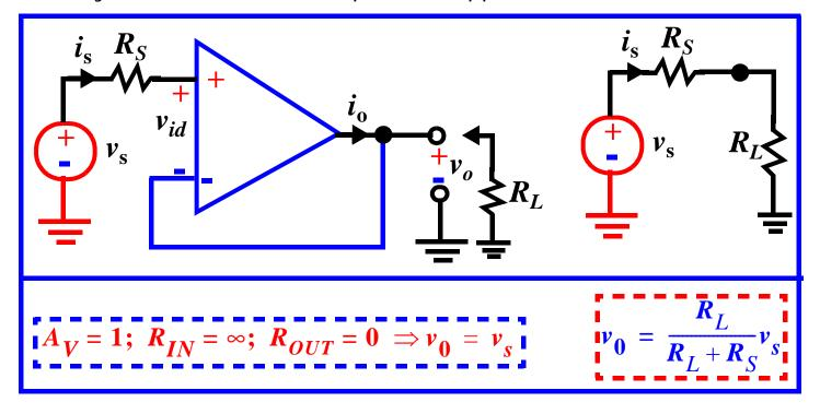
This is a resistance translator. The source delivers no current; dissipates no energy; current and energy absorbed by  $R_{L}$  is supplied by OA.
