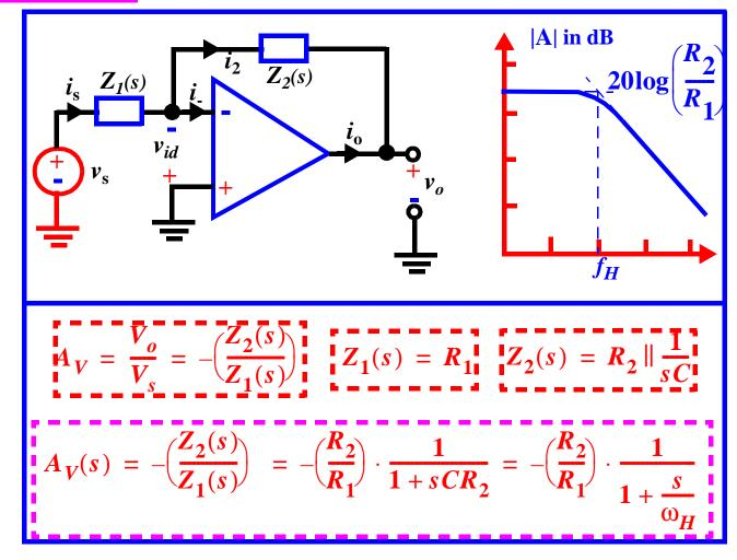
Two design parameters - low frequency gain and 3dB frequency can be set independently since we have 3 parameters -  $R_1$ ,  $R_2$  and C.
