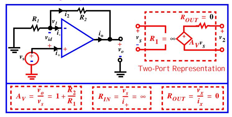
Now  $A_V$  depends only on the ratio of R's. This is important, e.g., R's can vary with temperature, but their ratio remains the same. That is, we can make a stable circuit using unstable components.
