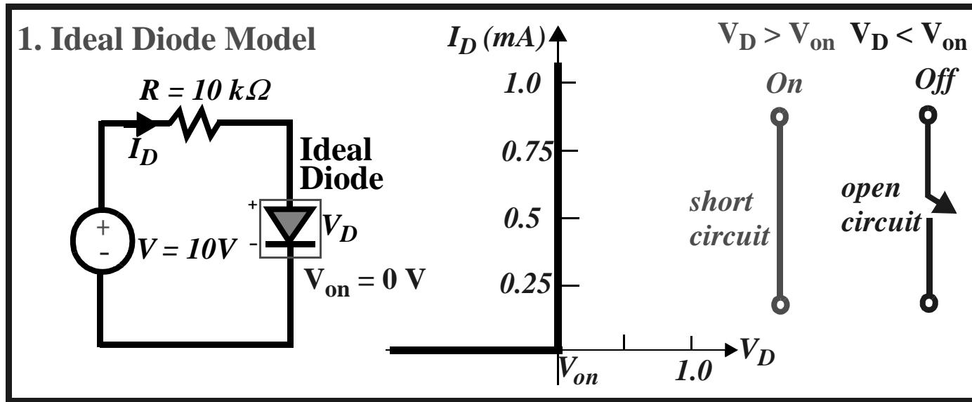
$$V_D = 0 \text{ for } I_D > 0 \text{ and } I_D = 0 \text{ for } V_D < 0.$$
