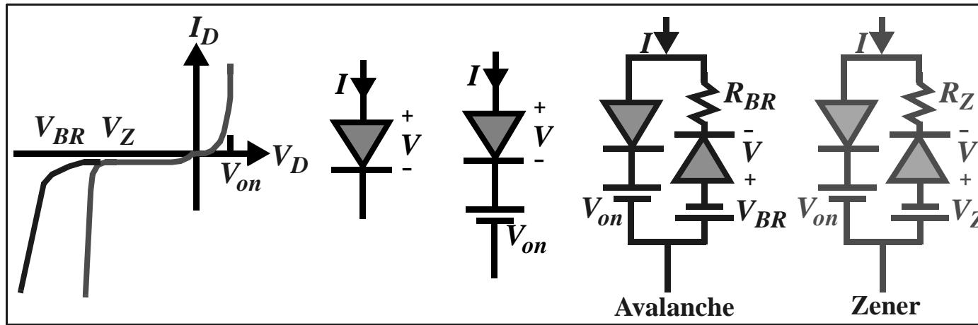
**Avalanche Breakdown** - occurs at high voltages  $V > V_Z$ . Here, carriers gain sufficient energy from E-field to knock electron-hole pairs from covalent bonds. Also  $V_Z$  increases as  $T$  increases.
