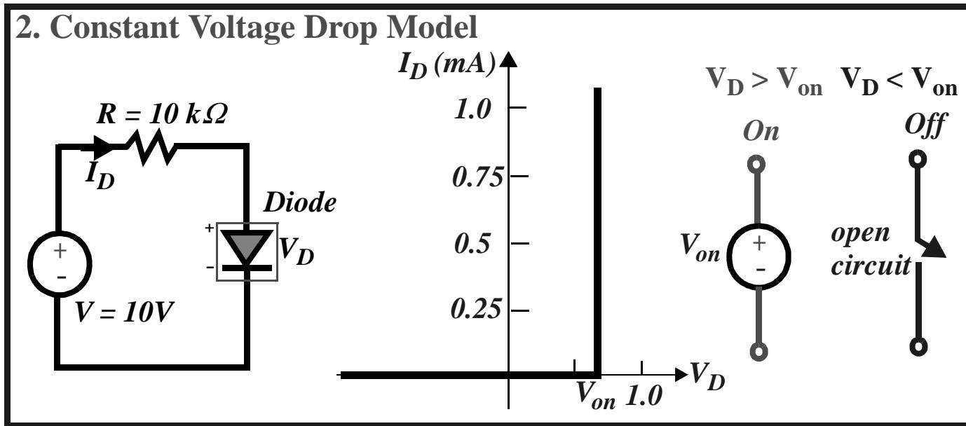
$$V_D = V_{on} \text{ for } I_D > 0 \text{ and } I_D = 0 \text{ for } V_D < V_{on}.$$
