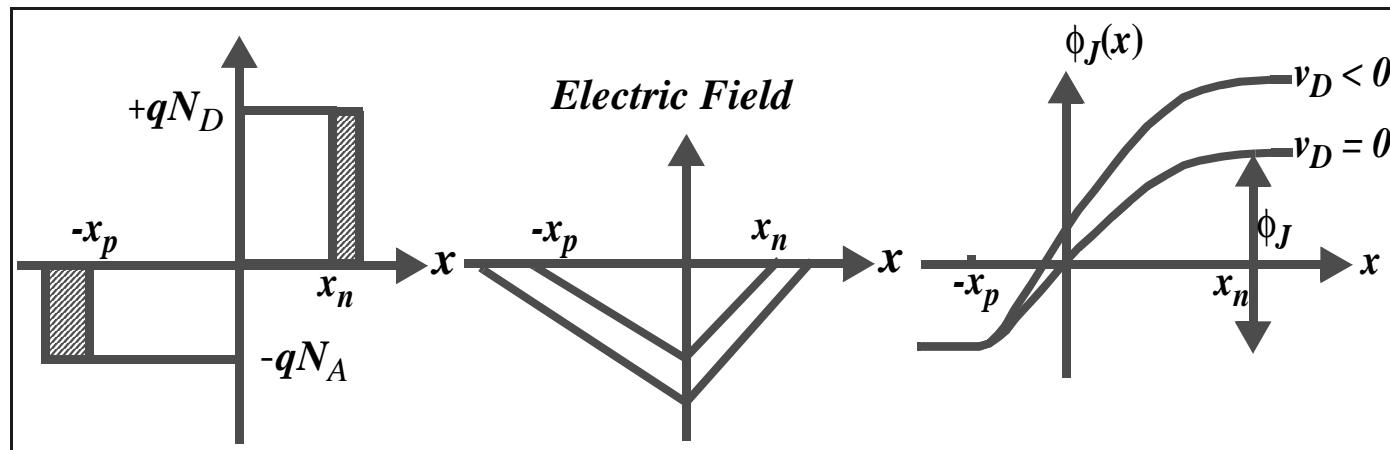
Zener Breakdown - occurs only in heavily doped diodes. The heavy doping results in narrow depletion regions. Reverse bias causes tunneling between **CB** and **VB** with **I** increasing rapidly. The breakdown voltage (**V<sub>Z</sub>**) can vary from a few volts to 100's of V. Zener diodes are used to maintain a constant **V** for varying **I**'s. Used in voltage regulators. Also **V<sub>Z</sub>** increases as **T** decreases.
