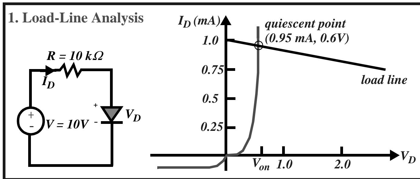
$$V = I_D R + V_D \quad . V_D = 0 \Rightarrow I_D = \frac{V}{R}; I_D = 0 \Rightarrow V_D = V$$
