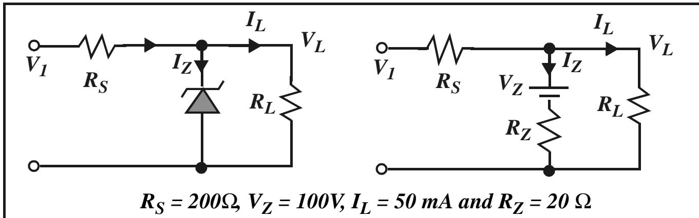
$$V_L = V_Z + I_Z \cdot R_Z = 100 + 0.01 \times 20 = 100.2V \quad . \quad I_Z = \frac{V_L - V_Z}{R_Z}$$
