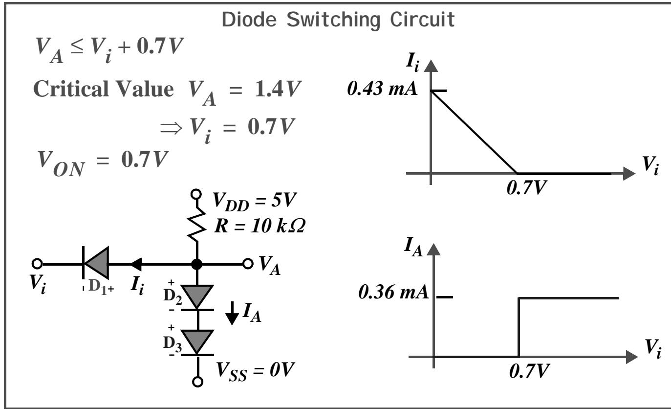
As an exercise, determine the value of  $V_A$  for the following values of input voltage  $V_i = 2V, 1V, 0V$  and  $-1V$ .
