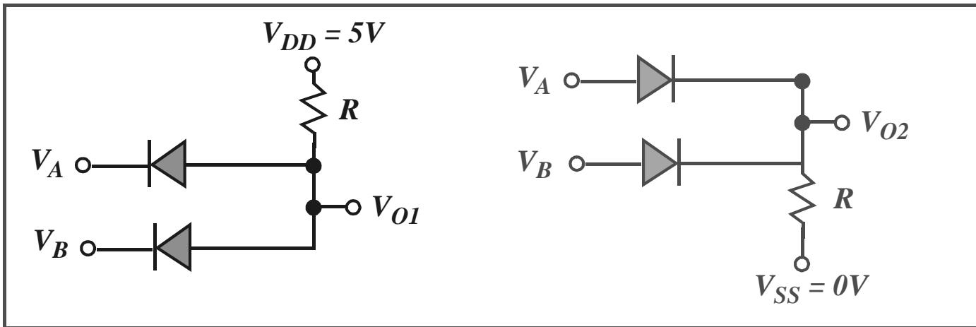
For the two circuits above, determine  $V_{O1}$  for all four combinations of  $V_A$  and  $V_B$ , of 0V and 5V, that is (0V,0V), (0V,5V), (5V,0V) and (5V,5V). How best can  $V_{O1}$  and  $V_{O2}$  be written in terms of  $V_A$  and  $V_B$ .
