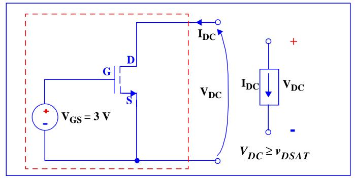
A depletion mode nMOSFET has  $V_{TN}$  = -2V,  $K_n$  = 4mA/V² and  $\lambda$  = 0V¹¹ and is used as a current source. Determine the voltage at the source S of M1.
