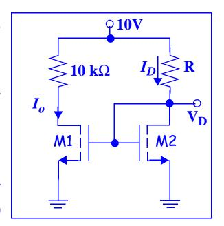
$\mu$ m, L = 10  $\mu$ m and  $\lambda$  = 0V<sup>-1</sup>. Can you generalize your result if the aspect rations (W/L) of M1 and M2 are different.
