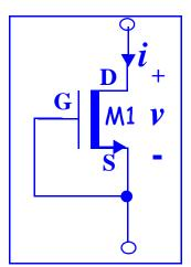
Design Problem. An enhancement mode nMOSFET is used to obtain a current of 0.4 mA. Its parameters are  $V_{TN}$  = 1V,  $K_n$  = 0.2mA/V², W = 100  $\mu$ m, L = 10  $\mu$ m and  $\lambda$  = 0V¹¹. Design a circuit that would perform as above, and determine its mode of operation. (Here, one design is the circuit shown on the right.)
