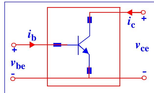
$$y_{11} = \left. \frac{\mathbf{i}_b}{\mathbf{v}_{be}} \right|_{\mathbf{v}_{ce} = 0} = \left. \frac{\partial i_B}{\partial v_{BE}} \right|_{Q-P}; \quad y_{12} = \left. \frac{\mathbf{i}_b}{\mathbf{v}_{ce}} \right|_{\mathbf{v}_{ce} = 0} = \left. \frac{\partial i_B}{\partial v_{CE}} \right|_{Q-P}$$
