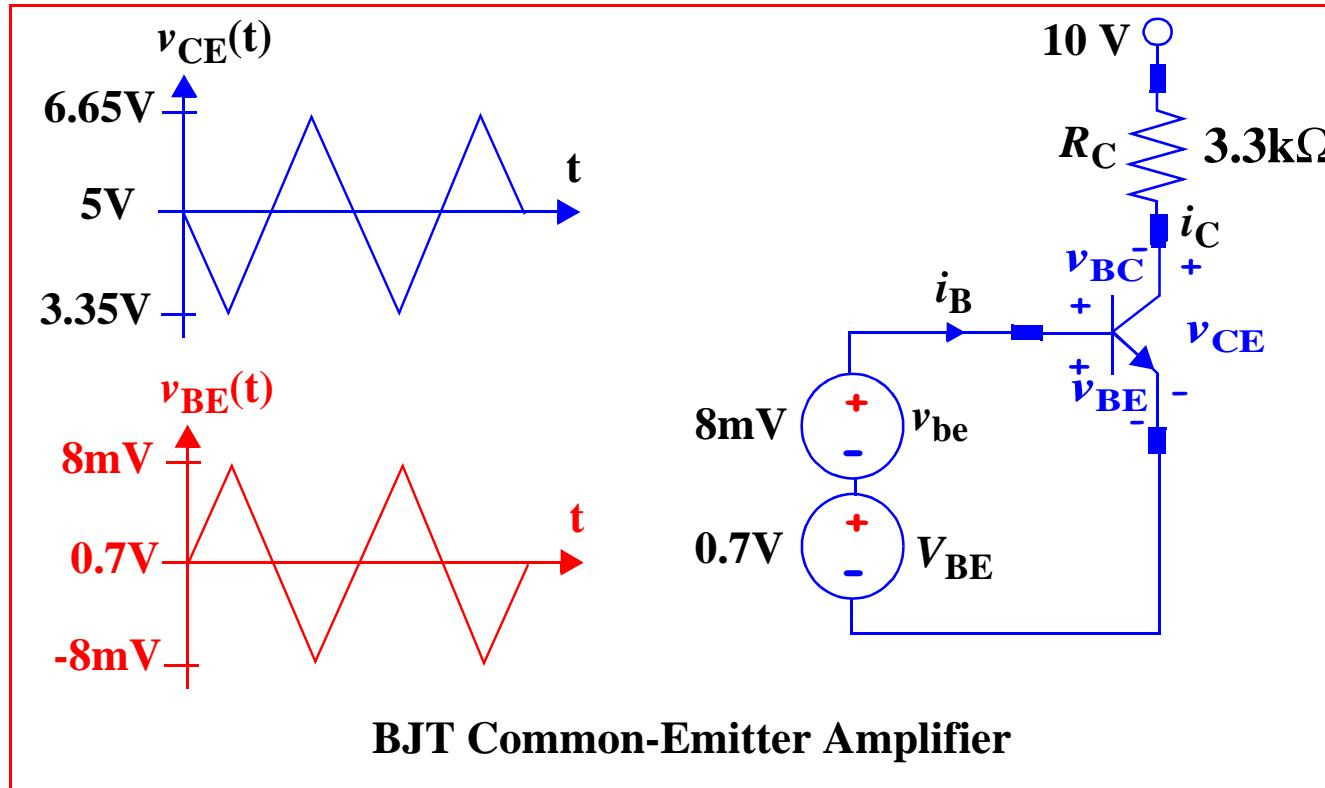
$i_B = 15\mu\text{A}$ ,  $i_C = 1.5\text{mA}$  since  $\beta = 100$
