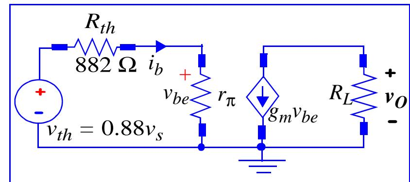
Final equivalent circuit of common-emitter amplifier.
