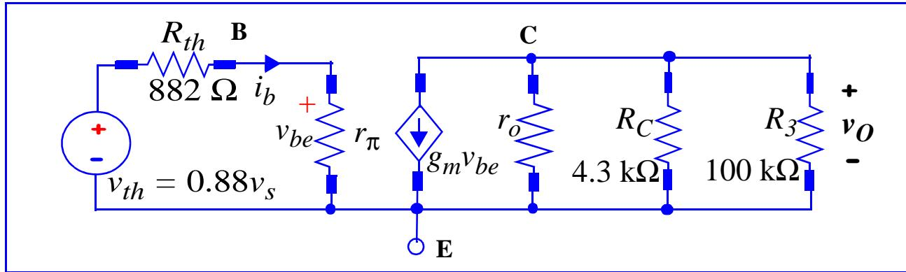
AC Equivalent Circuit with BJT replaced with its SS model.
