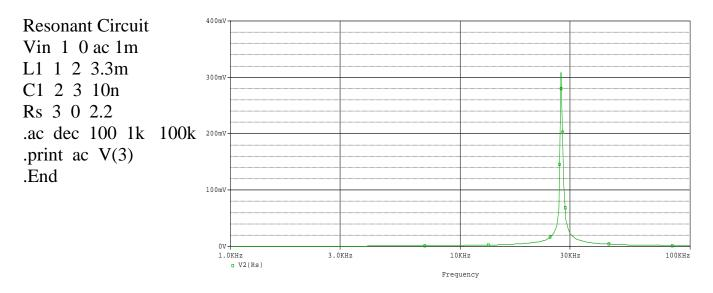
Other types of AC analysis are .Noise, .Disto and .pz. They carry out noise analysis, distortion analysis and pole-zero analysis of the circuit.
