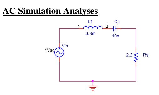
.AC directive enables a frequency sweep of the frequency
