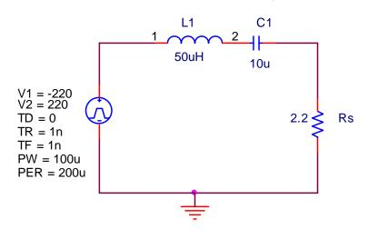
\* PULSE(-Vs Vs TDelay TRise TFall PulseWidth Period) Vin 1 0 PULSE(-220V 220V 0 1ns 1ns 100us 200us) L1 1 2 50u C1 2 3 10u Rs 3 0 2.2 .TRAN 1US 400US .Probe .END
