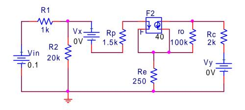
.TF directive obtains the transfer function between two sets of input pairs
