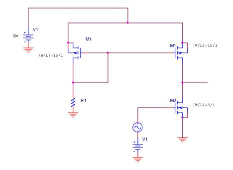
For the shown circuit we have  $V_{TN}=1.0 \text{ V}$ ,  $V_{TP}=-1.0 \text{ V}$ ,  $K_n=0.36 \text{ mA/V}^2$ ,  $K_p=25 \text{ e-6 A/V}^2$ a) Explain the theory of operation of the shown amplifier
