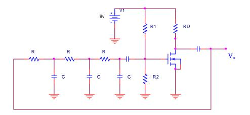
The above figure shows a sinusoidal oscillator utilizing an NMOS transistor. The transistor has the following parameters:  $V_{TN}$ =1.0V and  $K_n$ =1.0 mA/V<sup>2</sup>
