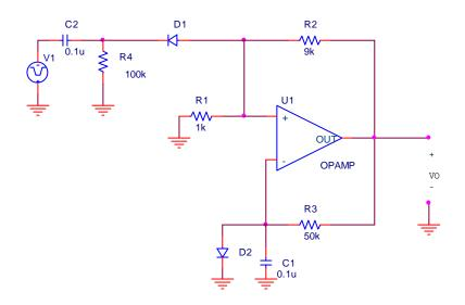
A monstable circuit is a circuit that generates a pulse of fixed duration in response to a trigger signal of any duration. The OpAmp in the above circuit is connected to a dual supply of +15 V and -15V.
