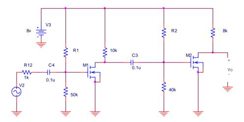
The MOSFETS in the above circuit are identical with  $K_n=1.6 \text{ mA/V}^2$ ,  $V_{TN}=0.8 \text{ V}$  and  $\lambda=0.018 \text{ V}^{-1}$ . Design the values of the resistors  $R_1$  and  $R_2$  so that the total gain of this two-stage amplifier is 110. Verify your design using PSpice.
