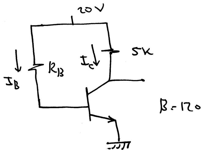
find  $R_B$  such that  $V_{CEQ} = 10V$
