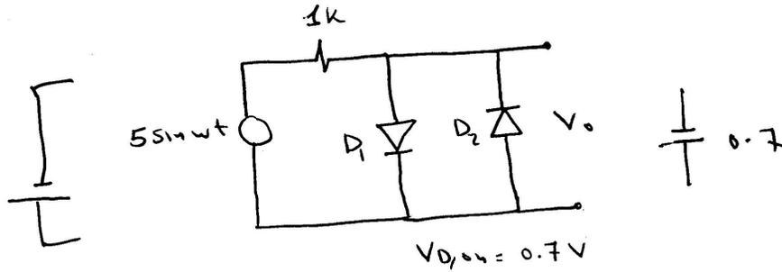
Express the output voltage as a function of the input voltage.
