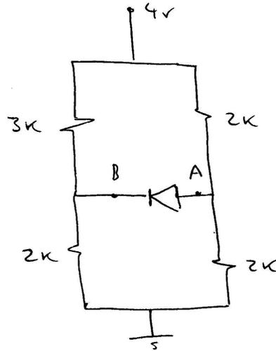
Find the Q-point for the shown diode using the ideal diode model and the CD model with  $V_{D,ON} = 0.6V$
