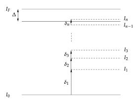
Fig. 12. A pictorial illustration of the modeled programming sequence. On the left side are the initial level  $I_0$ , the target level  $I_F$  and the tolerance parameter  $\Delta$ . In the middle is a sequence of exponentially distributed level increments  $\delta_1, \delta_2, \ldots, \delta_n$  resulting from the programming algorithm. On the right side are the instantaneous levels  $I_i$  until the process terminates at  $I_n$ .
