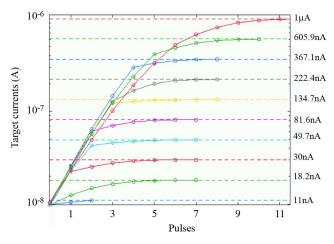
Fig. 10. Performance of a flash adaptive program sequence [3]. The circles on each curve describe the results of an iterative programming algorithm for a given target value.
