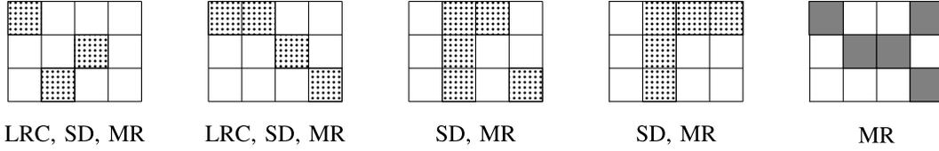
Fig. 1. Different types of erasure patterns recoverable for LRC, SD, and MR codes.
