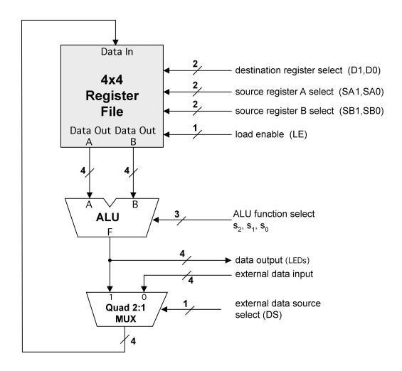
Using the graphic design editor, build this circuit using the previous components and compile, implement and test. This datapath has much more capability than our first design in Step 5:
