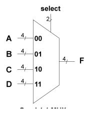
inputs, a 4-bit data output and two select lines as shown below. Study the VHDL source code given at the end of this lab that implements a Quad 4:1 multiplexer. Be sure you understand the logic of the VHDL code. Compile this program, implement and test using the MAX7000 device. Generate a symbol for this MUX which you will use later.
