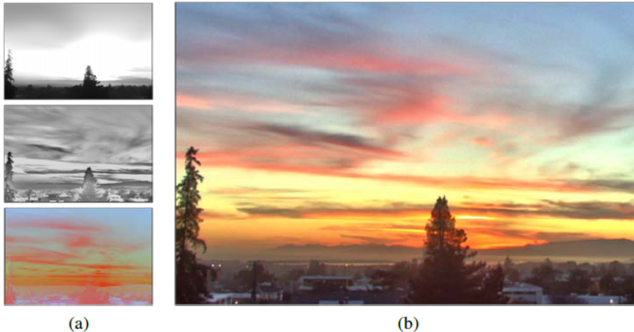
Figure 10.22 Local tone mapping using bilateral filter (Durand and Dorsey 2002): (a) low-pass and high-pass bilateral filtered log luminance images and color (chrominance) image; (b) resulting tone-mapped image (after attenuating the low-pass log luminance image) shows no halos. Processed images courtesy of Frédo Durand, MIT 6.815/6.865 course on Computational Photography.
