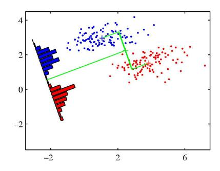
When projected onto the line joining the class means, the classes are not well separated.
