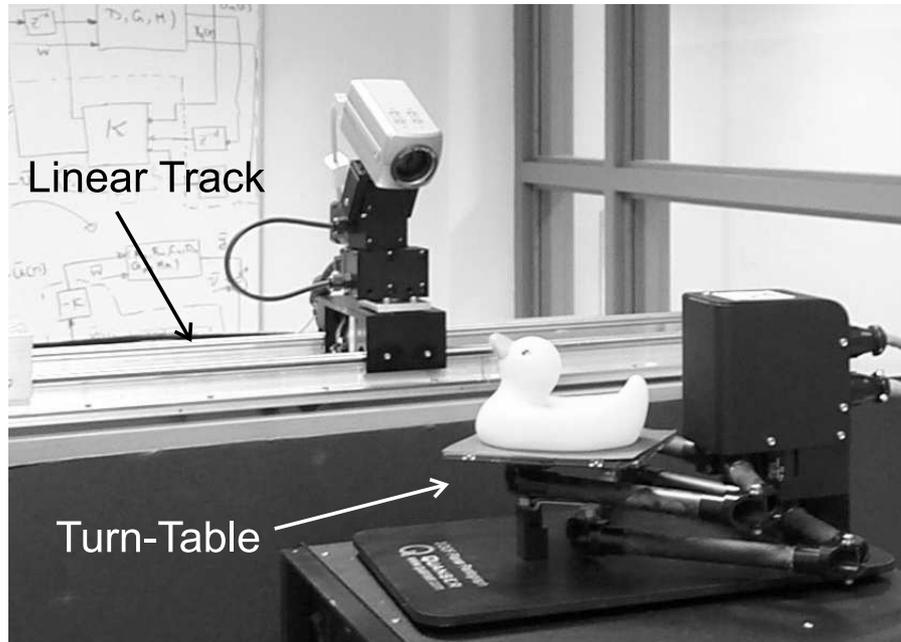
Figure 6.2: Camera 2 is positioned by a linear track; a twin pantograph unit serves as the turn-table.
