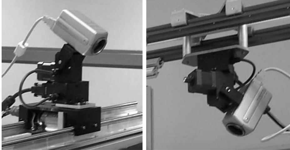
Figure 6.3: Pan-tilt units with the cameras attached; the left picture shows a sample positioning of Camera 2, whereas the picture on the right depicts the positioning of Camera 1.
