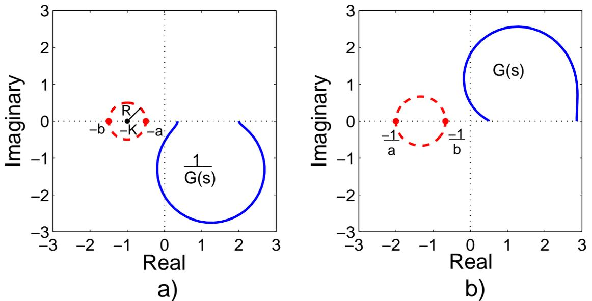
Figure 5.4: On-axis circle theorem test a) graphical interpretation of equation (5.20) b) transformed through  $z \mapsto 1/z$ . Here  $G(s) = \frac{s^2+6s+100}{0.35s^2+8s+200}$ ,  $a = 0.5$  and  $b = 1.5$ .
