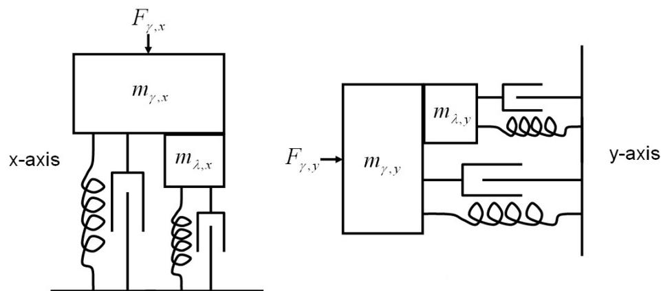
Figure 8.2: Dynamic model used for workspace controllers.
