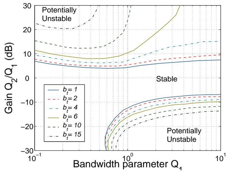
Figure 6.7: Notch position filter stability regions with  $\omega_n = 20\pi$  rad/s at different levels of virtual tool damping  $b_t$ .
