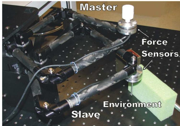
Figure 8.1: The two-axis experimental setup.
