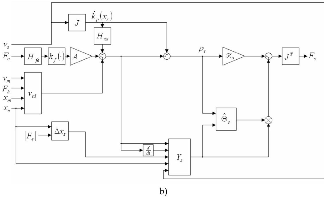
Figure 8.4: Adaptive controllers a) master controller b) slave controller
