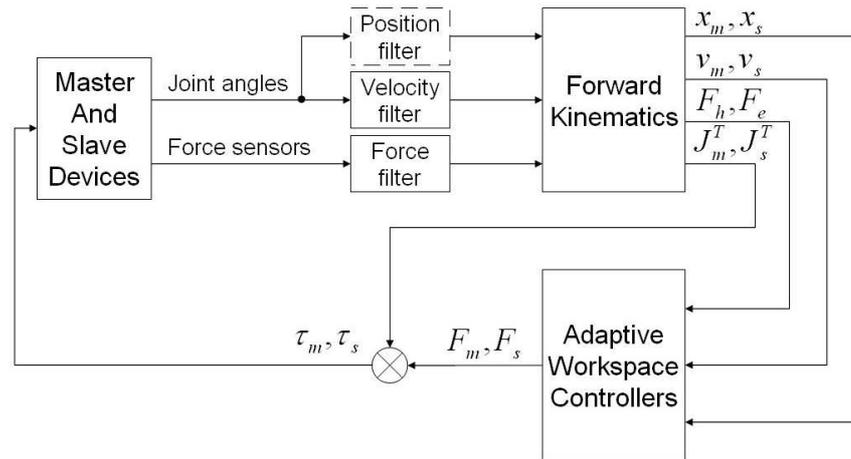
Figure 8.3: Control block diagram for teleoperation experiments.
