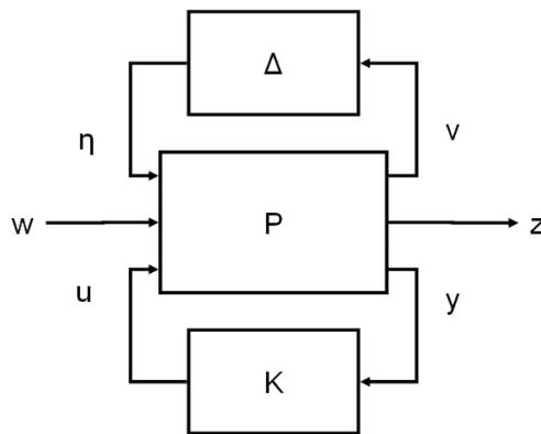
Figure 2.3: System for robust controller synthesis
