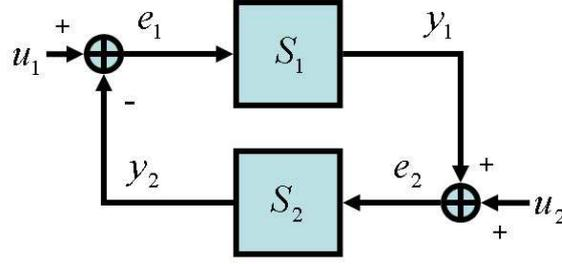
Figure 5.2: Passivity theorem block diagram.
