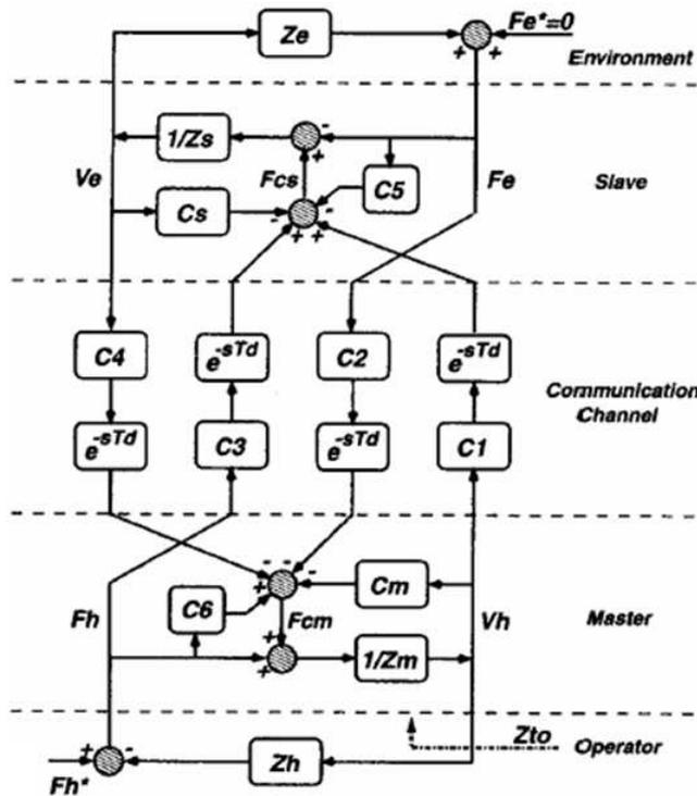
Figure 2.2: Teleoperation block diagram. Figure from [1].
