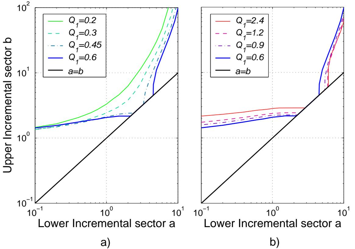
Figure 6.8: Stability regions from off-axis circle criterion with notch position filtering at  $\omega_n = 18\pi$  rad/s with gain  $\frac{Q_2}{Q_1} = 5$  and varying bandwidth. a)  $0.2 \leq Q_1 \leq 0.6$  b)  $0.6 \leq Q_1 \leq 2.4$ .
