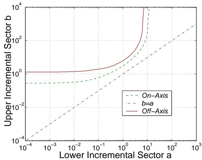
Figure 6.2: Off-axis vs. on-axis circle criterion: the stable region is between the straight and curved lines.
