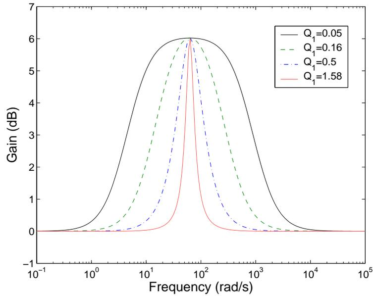
Figure 6.6: Position filter  $H'_{xs} = (s^2 + \frac{\omega_n}{Q_1}s + \omega_n^2)/(s^2 + \frac{\omega_n}{Q_2}s + \omega_n^2)$  with  $\omega_n = 20\pi$  rad/s,  $Q_2 = 2Q_1$  at different values of  $Q_1$ .
