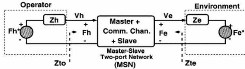
Figure 2.1: Teleoperation two port network model. Figure from [1].
