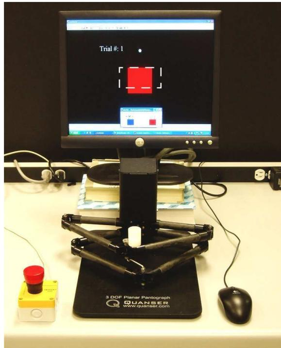
Figure 7.8: Setup for psychophysics experiments. Note: The dashed box represents the location of the selection dialog box under the haptics only experiments where visual feedback is removed.
