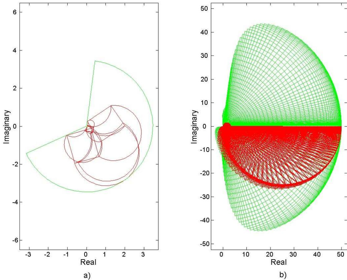
Figure 6.9: Nyquist overbounding a) Nyquist template at  $\omega = 30$  rad/s b) Nyquist envelopes. The overbounded Bode envelope approach is in lighter (green) colour whereas the true Nyquist envelope is in darker (red) colour.
