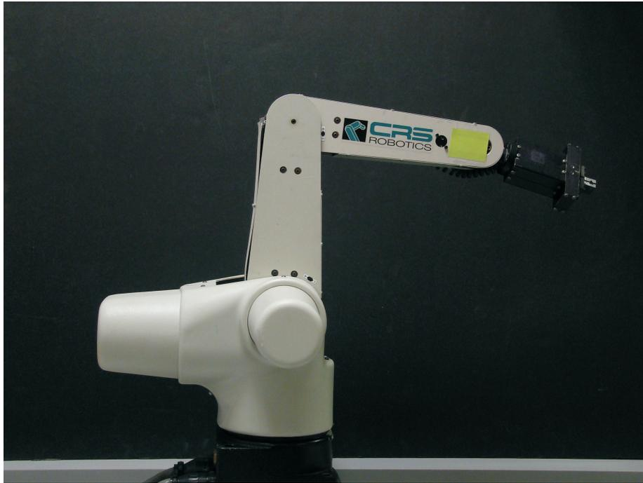
Figure 2.2: Open-chain robotic manipulator by CRS Robotics
