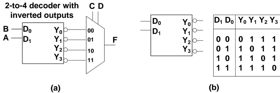
Figure 2 – (a) Circuit for question 5. (b) Truth table of the decoder with inverted outputs
