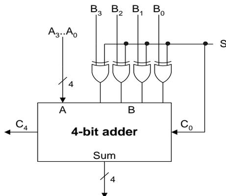
Figure 3 – Circuit for questions 7 to 11. Note,  $c_0$  is carry in and  $c_4$  is carry out for the 4-bit adder.
