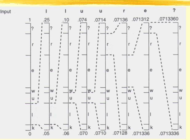
Final range is [0.0713336, 0.0713360). Transmit any number within range, e.g. 0.0713348389... **16 bits**. (Huffman coder needs 18bits. Fixed coder: 21bits). 4/11/2006
